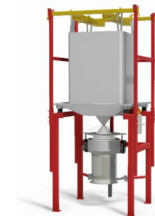
BAGBOY HYGIEN Gen. II type B Floor stand (10b) with bag support (4b), bag suspension rack (1b) and yoke for truck or crane (18c). Clamping unit (21) for fixing and stretching of emptying nozzle, controlled from a pneumatic control cabinet (20).
