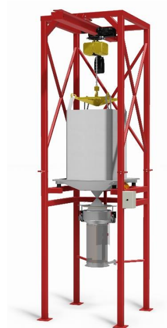
BAGBOY HYGIEN Gen. II type C Traverse stand (10c) with bag support (4b), electric chain hoists (17) and lift (18a). Clamping unit (21) for fixing, stretching and emptying of the nozzle, controlled from a pneumatic control cabinet (20).
