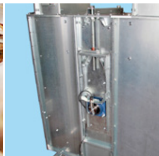
Belt tension in boot & speed monitor.
