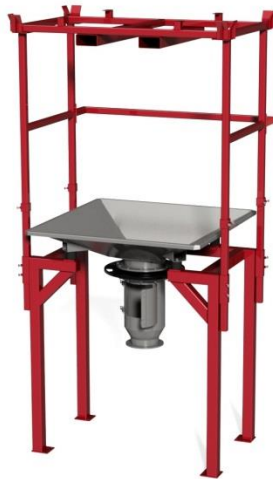
BAGBOY HATCH type B Floor stand (10b) with sack support (4b), bag suspension rack (1b) and yoke for truck or crane (18c). Iris damper (23) and door part (22) for opening of emptying nozzle.
