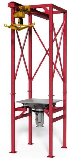
BAGBOY HATCH type C Traverse stand (10c) with sack support (4b), electric chain hoists (17) and lift (18a). Iris damper (23) and door part (22) for opening the drain nozzle.
