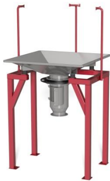
BAGBOY HATCH type A Floor stand (10a) with sack support (4b) and with centering arms (1a). Iris damper (23) and door part (22) for opening of emptying nozzle.
