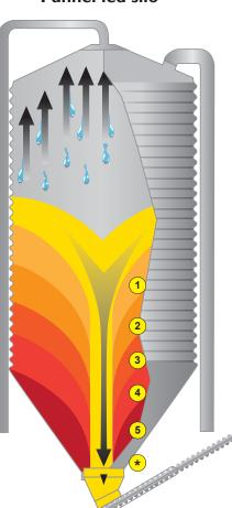
The silo cannot be completely filled up - unused capacity.
